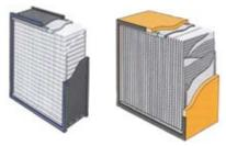
Esco cabinets use Swedish Camfil Farr® mini-pleat filters without aluminum separators to increase filter efficiency, minimize the chance of leakage, and to prolong filter life. Filters include a lightweight aluminum frame for structural stability and elimination of swelling common to conventional wood frames.
