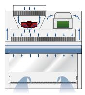
1C: If the exhaust fan fails (1c), the supply fan continues to provide inflow to the cabinet and downflow to the work area. The control panel warns of inflow failure.
