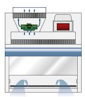
**1B:** If the supply fan fails (1b), downflow to the work area is suspended. The exhaust fan still provide inflow to the cabinet to help maintain containment. The control panel warns of downflow
