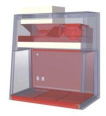
The Esco v-wall creates a Dynamic Chamber plenum which surrounds contaminated areas with negative pressure, preventing the possibility of contamination from leaks in filter seal, gasket or cabinet structure.
